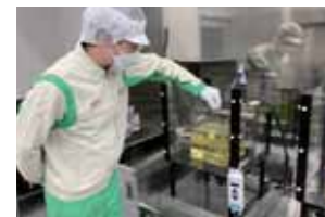
A glass fryer allows for checking the degree of frying from every angle
